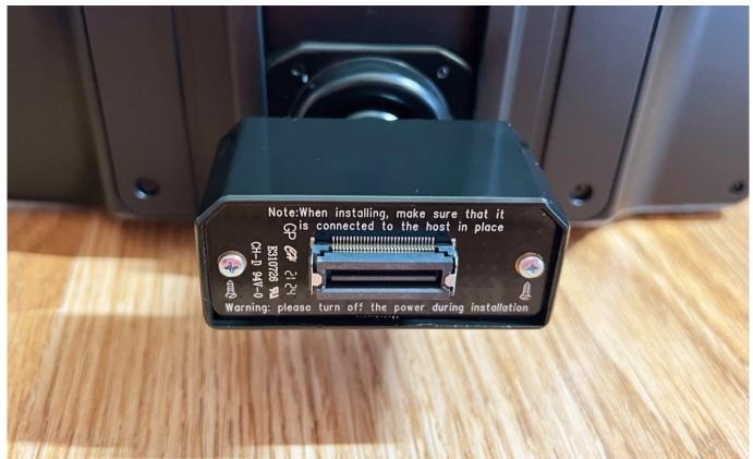
The connector at the back of the display, used to plug into the head unit itself.
