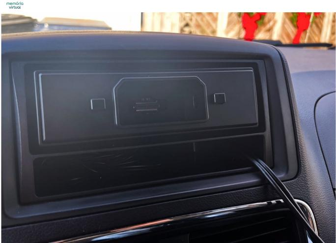
The head unit just shows the port where the display attaches once installed.
